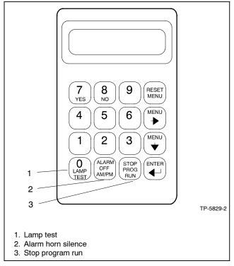
Figure 1-8 Keypad Switches
